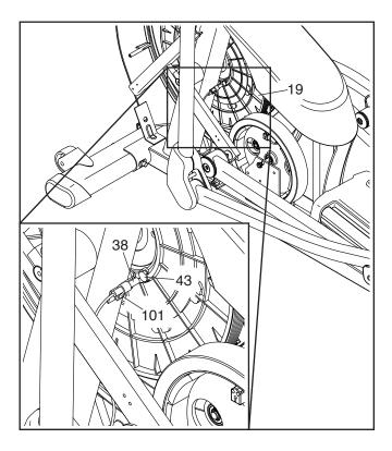
Slightly loosen the indicated M4 x 16mm Screw (101). Slide the Reed Switch (38) slightly closer to or away from the Magnet (43), and then retighten the Screw.
